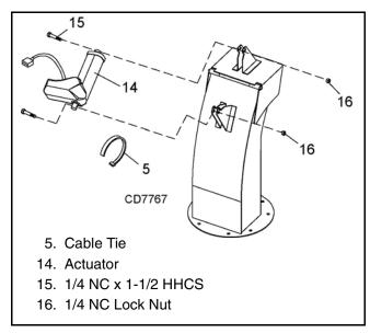
Figure 18. Electric Chute Deflector Installation
